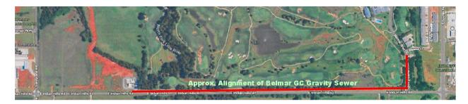
Belmar Gravity Line pipe alignment was evaluated in the Engineering Report prepared by Eagle Consultants, Inc. The alignment shown above will be further refined in collaboration with City of Moore. After the alignment has been finalized, the Consultant will provide all ground topographic and land tie surveying as required for the design of the project. Right-of-way has already been acquired by the City of Moore.
