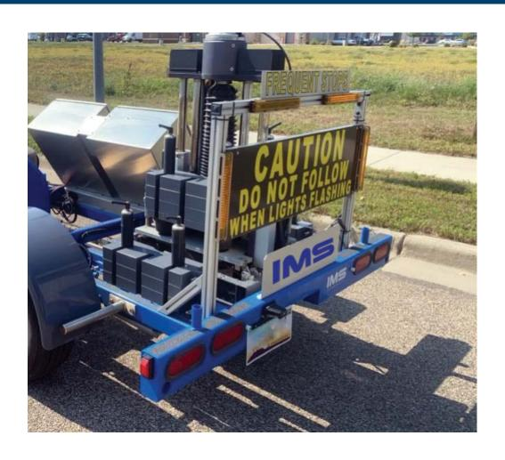
The FastFWD is a state-of-the art non-destructive tool used to perform structural testing. The purpose of this testing is to assess the load carrying capacity of a roadway or parking lot pavement to assess the remaining service life and determine the best rehabilitation strategy.
